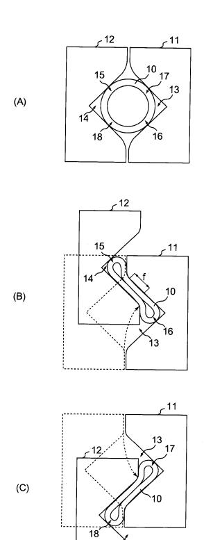
The present invention provides such pumping apparatuses that have very little deviation and high stability in pumping flow. A pumping apparatus comprises two opposing members (11, 12) that are set along a longitudinal direction of a tube (10) made of an elastic material with a relation that the space formed by grooves (13, 14) made in the two members (11,
