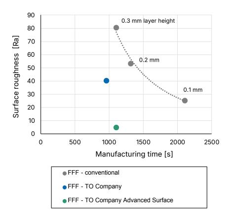
Comparing the surface roughness and manufacturing time, the software produces a higher surface quality at a shorter production time.
